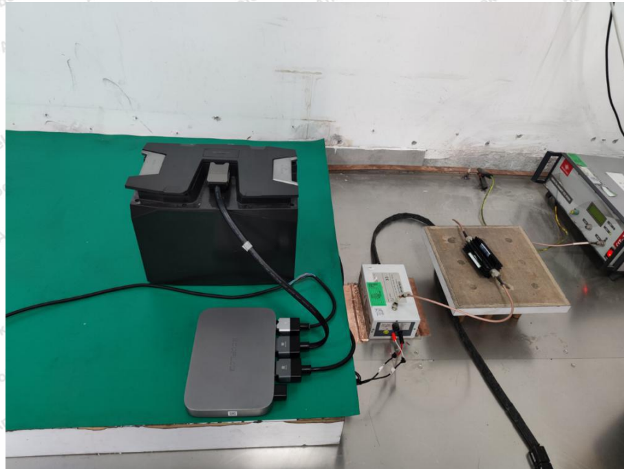
Photo of Injected Currents Susceptibility Test
