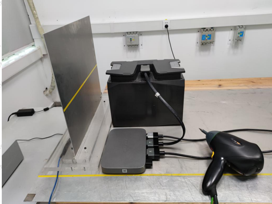
Photo of Electrostatic Discharge Immunity Test
