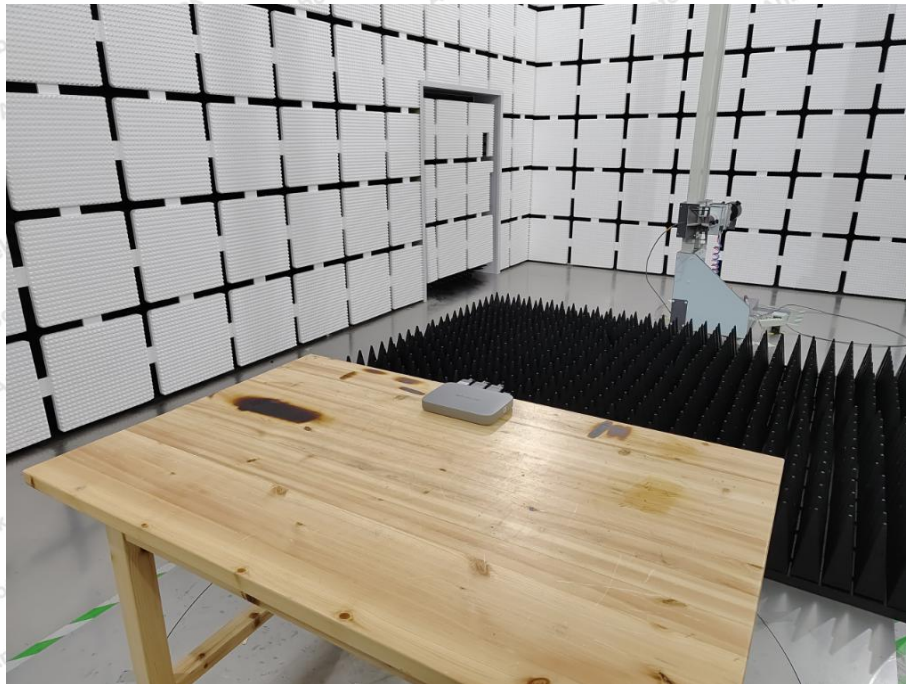
Photo of Radiated Emission Test (Below 1 GHz)
