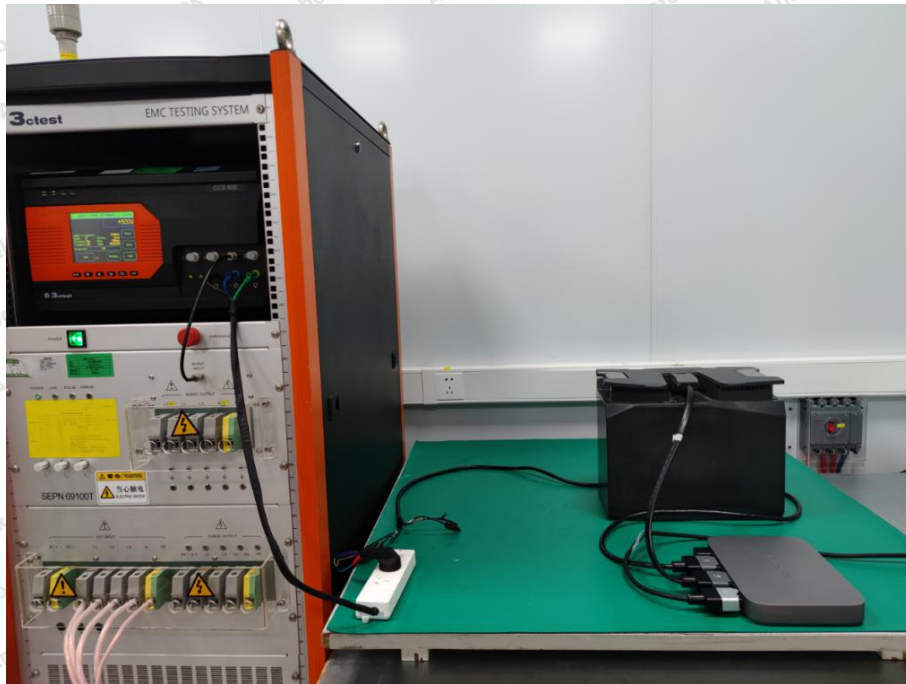
Photo of Electrical Fast Transient/Burst Immunity Test
